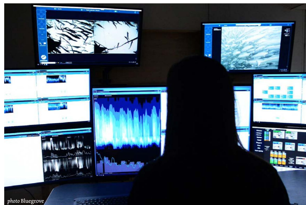
Pellet detection software at work in a salmon cage.
